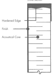
Avanti acoustical wall panel, 1" thick fabric finish, No. 4 (modified) mounting.
